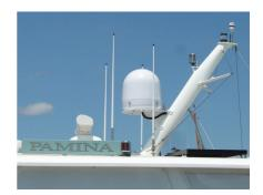
Use stainless steel fasteners, clamshell covers, and marine grade silicone where any exterior holes are drilled to prevent water intrusion.
