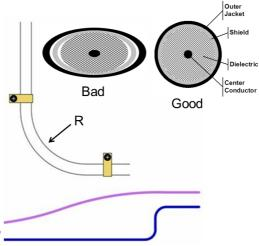
route coaxial cables using gentle S-curves
